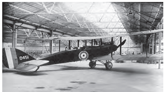
The first orders from the Air Ministry were for the De Havilland DH9 bomber. The first of the DH9s, D451 is nearing completion in March 1918
